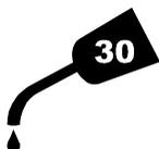
Lubricate with SAE 30 API-CD oil in intervals of recommended hours.
