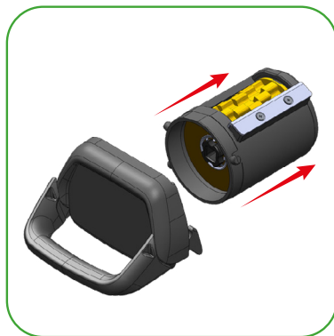
05 | Remova a calha.
